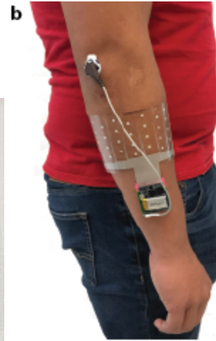
Figure 9. Electrode array built by UC Berkeley researchers and placement on arm [17]
